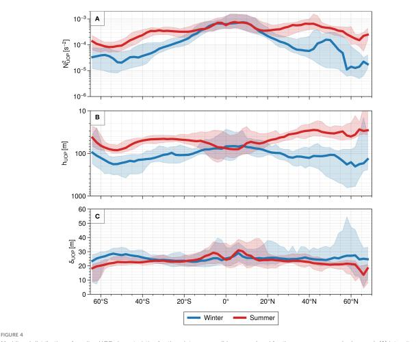
Meridional distribution of median UOP characteristics for the winter season (blue curves) and for the summer season (red curves): (A) intensity  $N_{UOP}^2$ , (B) depth  $h_{UOP}$  and (C) thickness  $\delta_{UOP}$ . The shaded areas represent the amplitude of the distributions within each zonal band based on the 5 and 95 percentiles.
