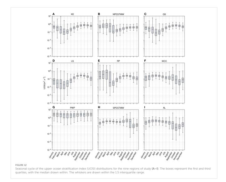
the median UOSI is small but the variability levels remain substantial all year long, with amplitude ratio comprised between those noticed for summer and those noticed for winter at higher latitudes. In this region, no restratification phase may be noticed as the UOSI remains large.
