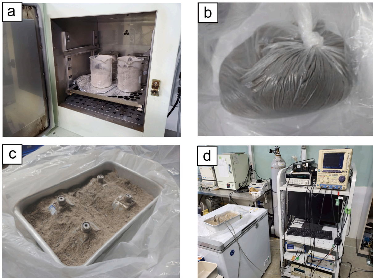
Fig. A1. Pictures of laboratory experiment. (a) Dry the lunar regolith simulant in oven. (b) Add certain amount of water mixed the certain amount of water and regolith simulant in the plastic bag. (c) Deploy the transducers of P-wave and S-wave within the regolith simulant. (d) The regolith simulant outside of the
