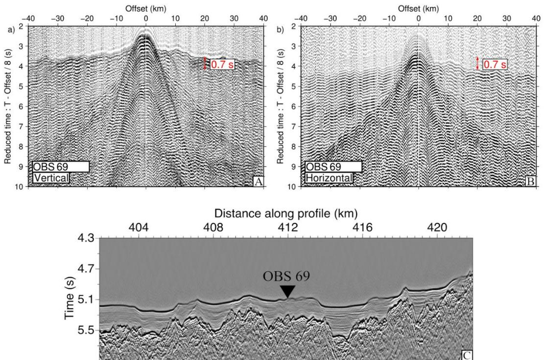
**Figure S6:** A) Vertical component of seismic data at OBS 69, B) horizontal component. The distance is from the OBS location. The sediment delay is marked. C) MCS image showing the location of OBS 69 along Profile 2.
