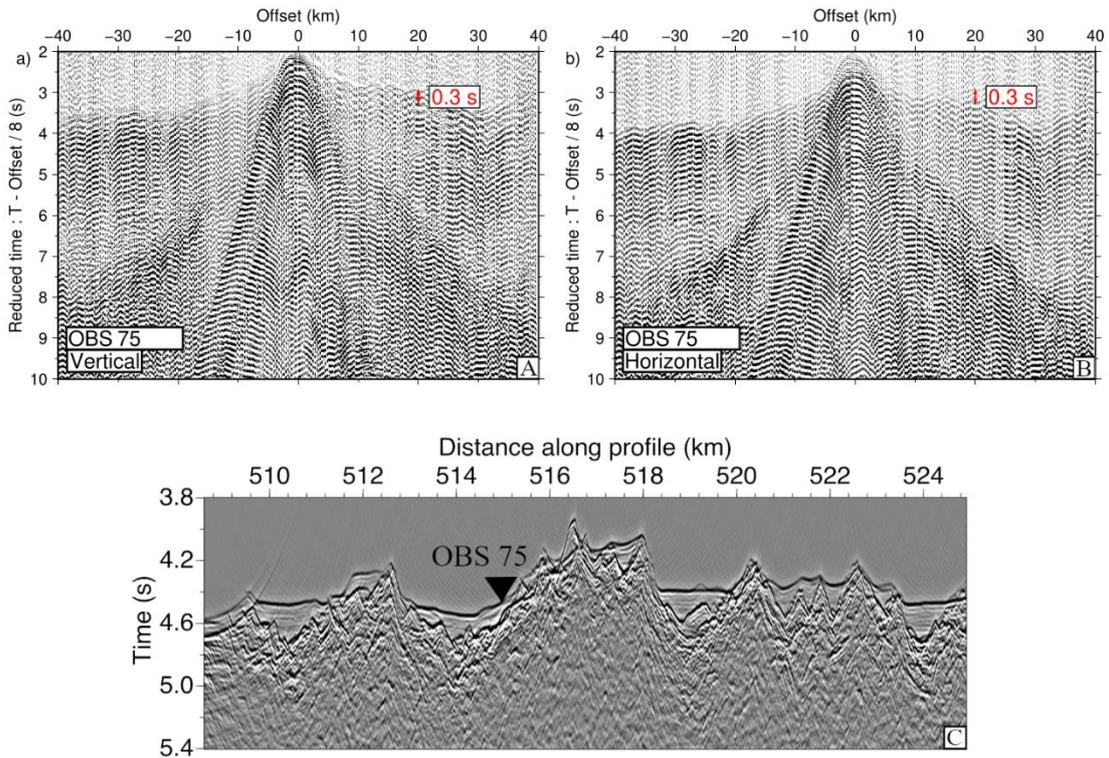
**Figure S7:** A) Vertical component of seismic data at OBS 75, B) horizontal component. The distance is from the OBS location. The sediment delay is marked. C) MCS image showing the location of OBS 75 along Profile 2.
