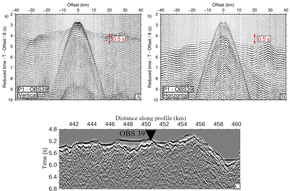
**Figure S3:** A) Vertical component of seismic data at OBS 39, B) horizontal component. The distance is from the OBS location. The sediment delay is marked. C) MCS image showing the location of OBS 39 along Profile 1.
