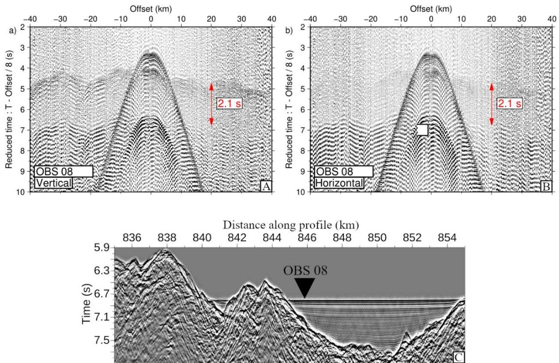
**Figure S1:** A) Vertical component of seismic data at OBS 08, B) horizontal component. The distance is from the OBS location. The sediment delay is marked. C) MCS image showing the location of OBS 08 along Profile 1.
