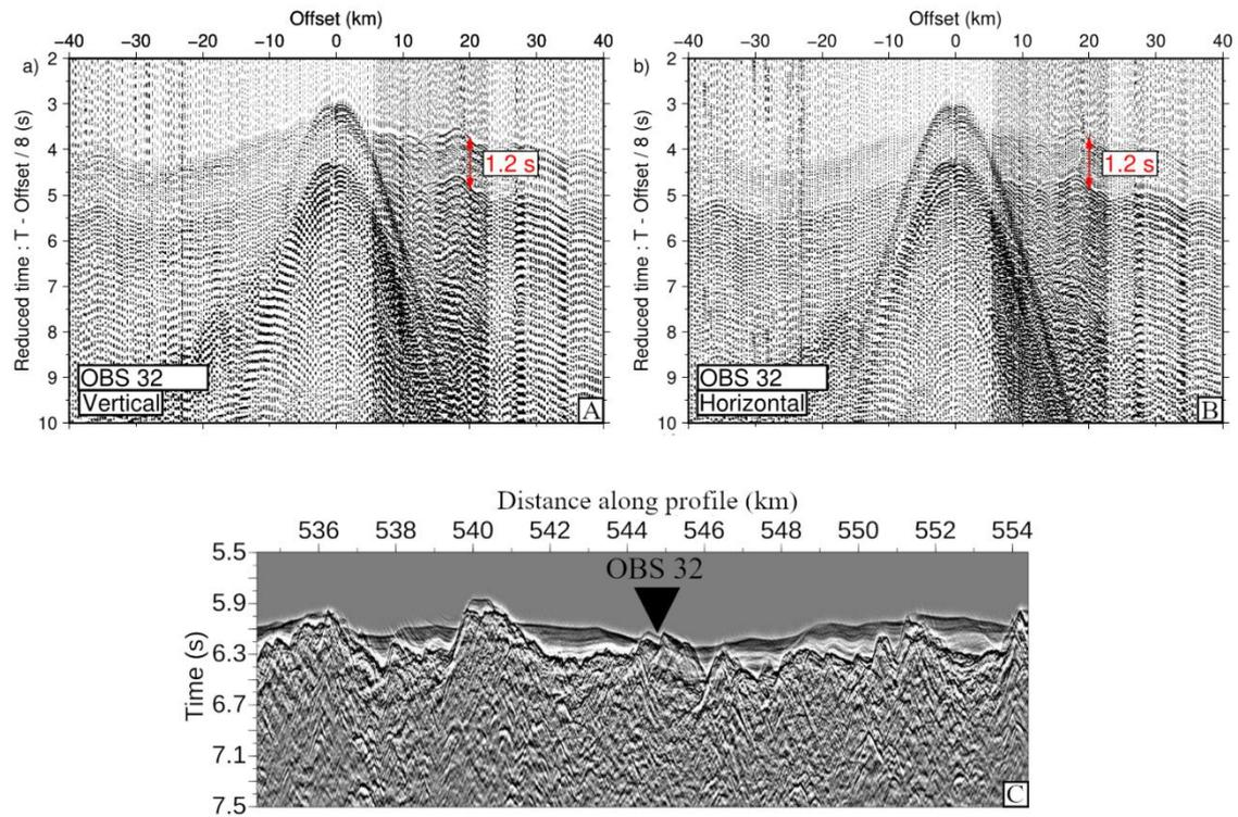
**Figure S2:** A) Vertical component of seismic data at OBS 32, B) horizontal component. The distance is from the OBS location. The sediment delay is marked. C) MCS image showing the location of OBS 32 along Profile 1.
