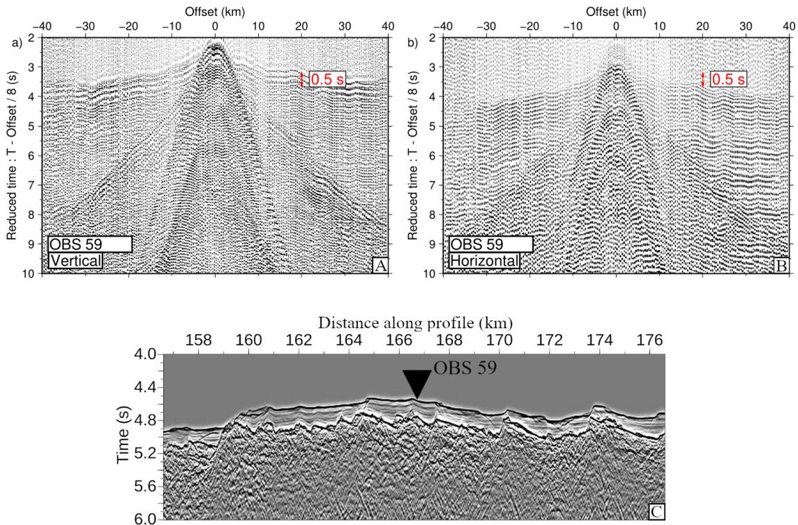
**Figure S4:** A) Vertical component of seismic data at OBS 59, B) horizontal component. The distance is from the OBS location. The sediment delay is marked. C) MCS image showing the location of OBS 59 along Profile 1.
