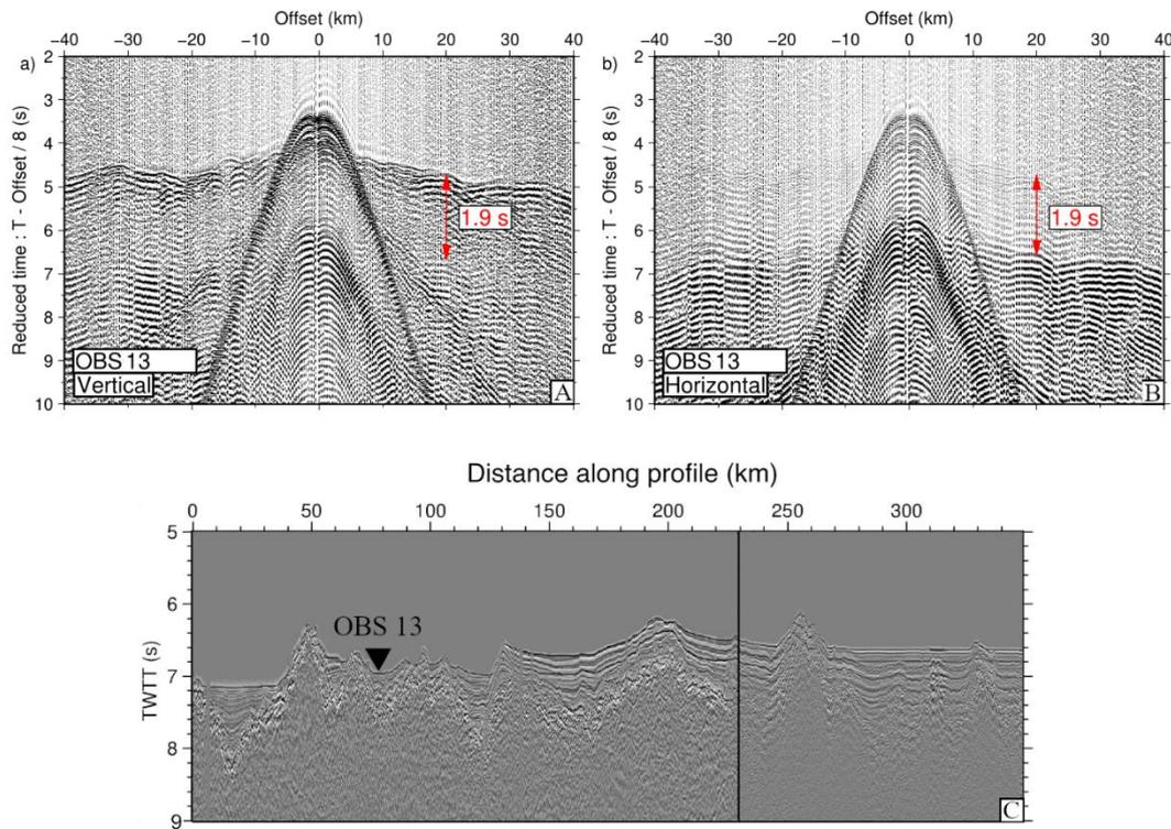
**Figure S10:** A) Vertical component of seismic data at OBS 13, B) horizontal component. The distance is from the OBS location. The sediment delay is marked. C) MCS image showing the location of OBS 13 along Profile 3 (modified from Grove et al., 2021).
