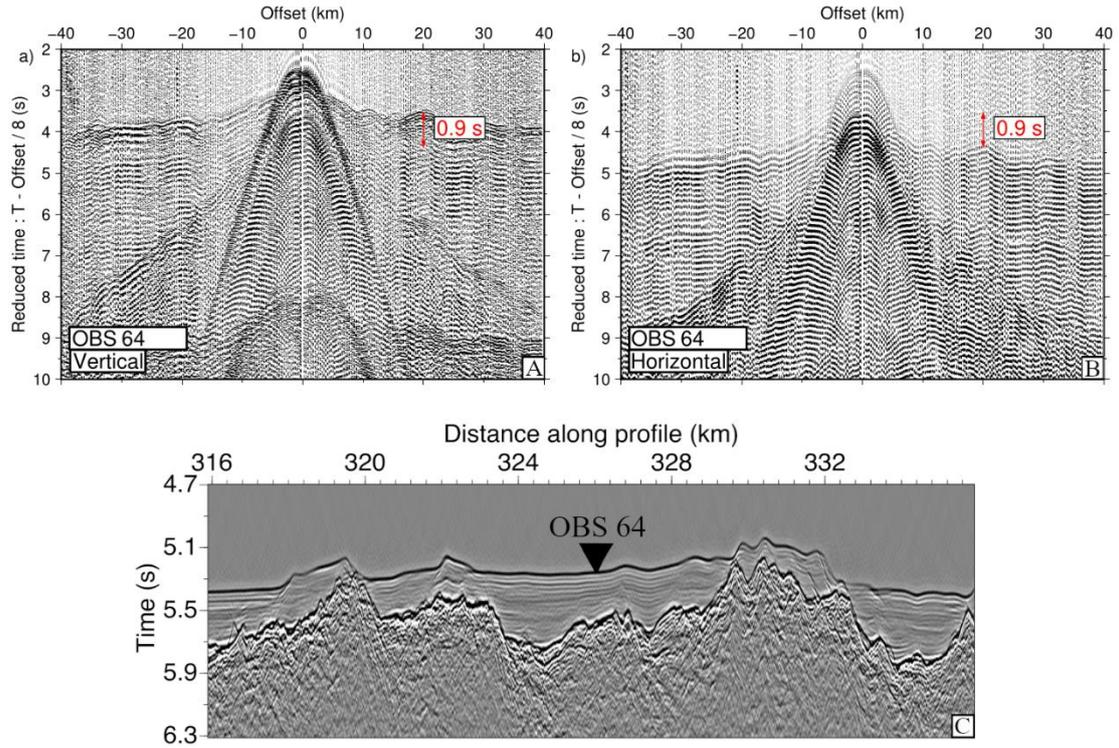
**Figure S5:** A) Vertical component of seismic data at OBS 64, B) horizontal component. The distance is from the OBS location. The sediment delay is marked. C) MCS image showing the location of OBS 64 along Profile 2.
