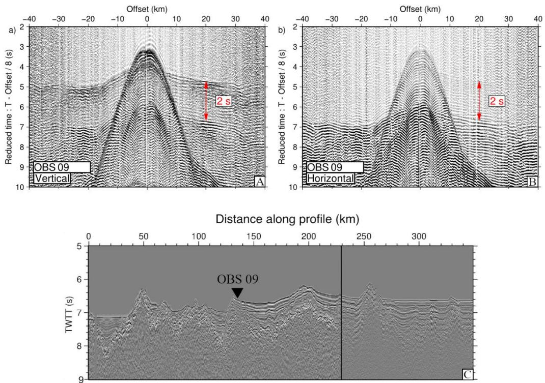
**Figure S9:** A) Vertical component of seismic data at OBS 09, B) horizontal component. The distance is from the OBS location. The sediment delay is marked. C) MCS image showing the location of OBS 09 along Profile 3 (modified from Grove et al., 2021).
