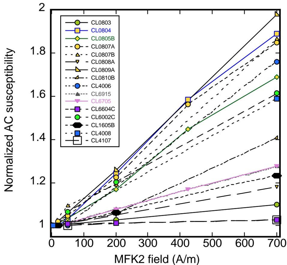
**Fig. 2.** Variation of the magnetic susceptibility versus the peak magnetic field available with the MFK2 instrument. Values are normalized to the one acquired at the lowest used field  $\leq 50$  A/m. Samples are from the set of Holocene volcanic rocks.
