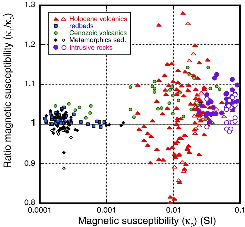
**Fig. 1.** Ratio  $\kappa_0/\kappa_1$  of the magnetic susceptibility (KLY3 instrument) after application of an IRM (filled symbols) or after AF demagnetization (open symbols) ( $\kappa_1$ ) to the susceptibility at the initial state ( $\kappa_0$ ) versus  $\kappa_0$ .
