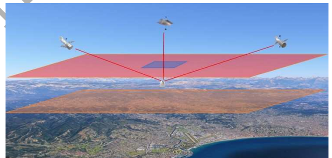
Figure 2. High spatial resolution (small rectangle 10\text{km} \times 10\text{km} ) vs. low spatial resolution (wide rectangle 100\text{km} \times 100\text{km} ) coverage comparison at Calern. Figure shows that the use of the high spatial resolution is not sufficient in the case of a partially covered sky.
