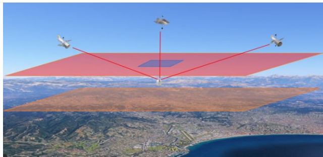
Figure 2. High spatial resolution (small rectangle 10 km × 10 km) versus low spatial resolution (wide rectangle 100 km × 100 km) coverage comparison at Calern. Figure shows that the use of the high spatial resolution is not sufficient in the case of a partially covered sky.
