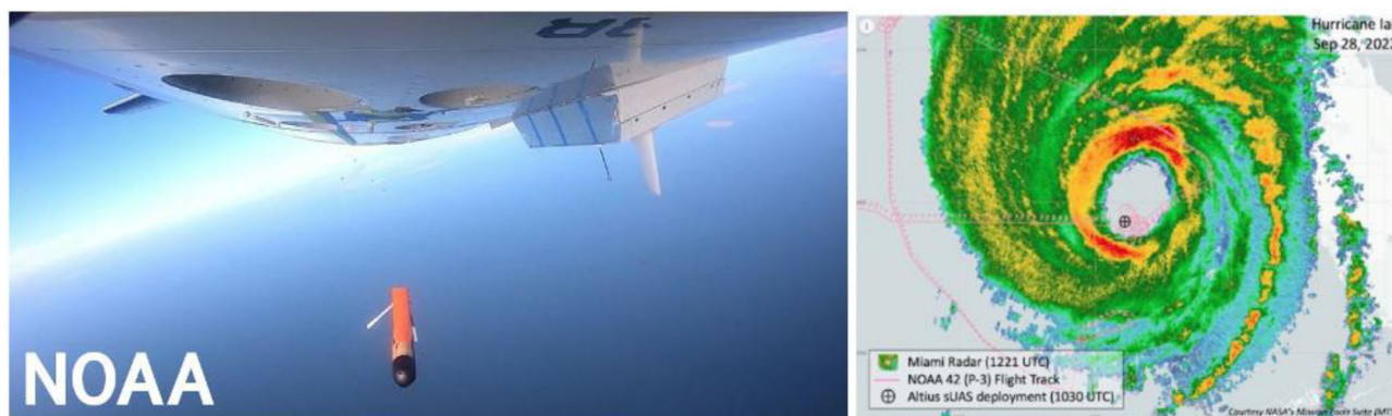
Fig. 11. (a) The Area-I's Altius 600 sUAS being deployed from one of the two NOAA P-3 aircraft. (b) Location of the drone into the eye of Hurricane Ian superimposed on radar reflectivity on September 28, 2022. Credit: NOAA.
