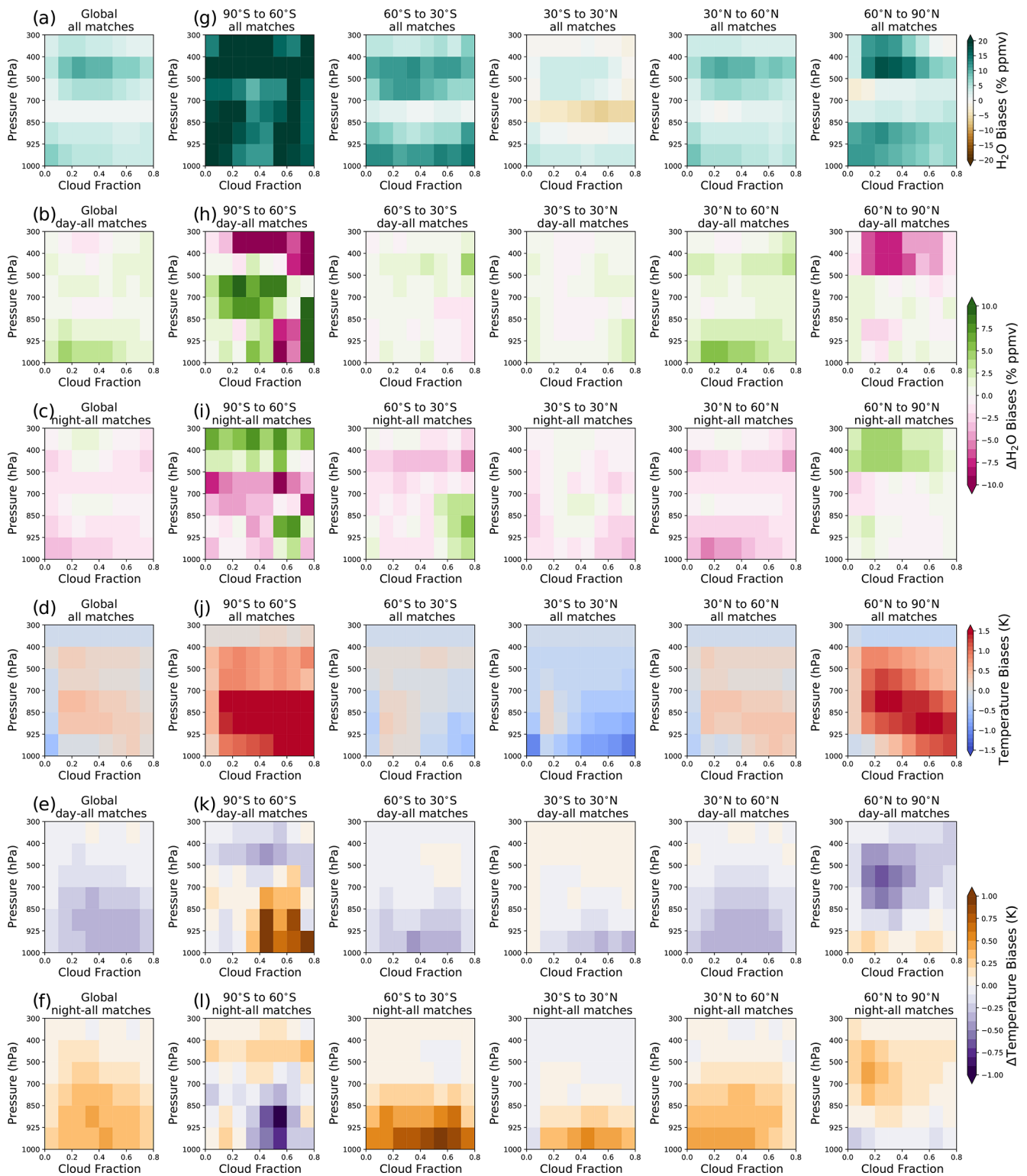
Figure 11. Cloud fraction effects on IMS biases relative to ARSA radiosonde water vapour and temperature profiles. Results here are broken down into global water vapour and temperature biases (a, d), daytime differences from global biases (b, e), night-time water vapour and temperature bias differences (c, f), and biases calculated for five broad latitudinal bands (g, j), as well as the daytime and night-time differences (h, i and k, l, respectively).
