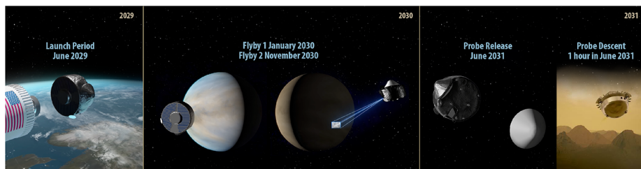
Fig. 11 DAVINCI offers definitive measurements from the top of the Venus cloud deck to the surface, while observing cloud dynamics and regional composition of key highlands including Alpha Regio. The Figure shows the nominal launch in June 2029; after a \sim 6 -month cruise, the spacecraft would fly by Venus in January 2030 for initial remote sensing in the UV and near-IR, then the trajectory returns 9 months later for a second flyby in November 2030. Both flybys will include dayside UV imaging and spectroscopy, as well as night side near-IR surface emissivity mapping of multiple tesserae including Alpha Regio. After an additional 7-month cruise, the flight system will deliver the probe in June 2031 for its entry, descent, and science campaign above western Alpha Regio at very high solar illumination conditions
