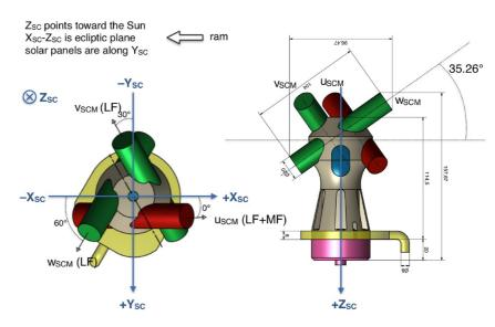
Figure B1. Schematics of the search-coil magnetometer and of the relation between its reference frame (u,v,w) and the one of the spacecraft (X,Y,Z).
