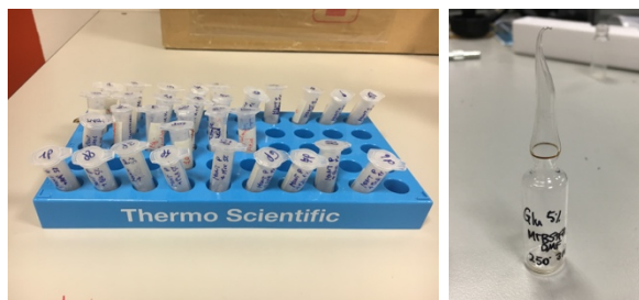
Figure 1: (Left) Montmorillonite samples spiked with organic molecules. Right) a sample sealed with 15 µL of MTBSTFA for MOMA-like derivatization.
