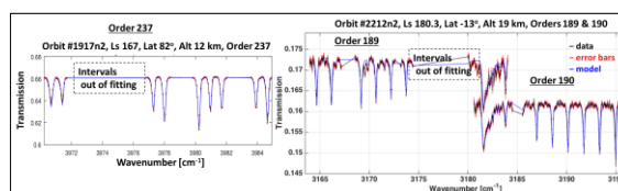
Figure 1: Examples of ACS-MIR spectral windows in diffraction orders 237 at 2.51 \mu\text{m} (left), and 189–190 at 3.15 \mu\text{m} (right), measured at tangent heights 12 and 19 km, used for the retrieval of \text{CO}_2 density.
