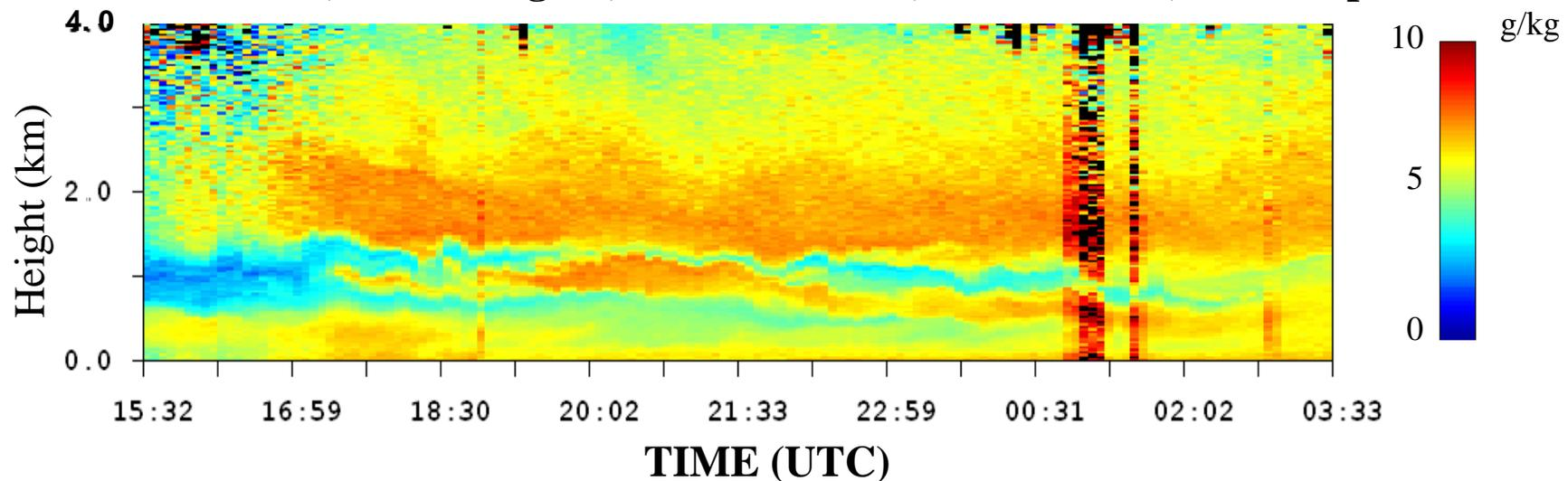
Measurements carried out by BASIL on 28 September 2012 reveal a **water vapour field** characterized by a **quite complex vertical structure**.
