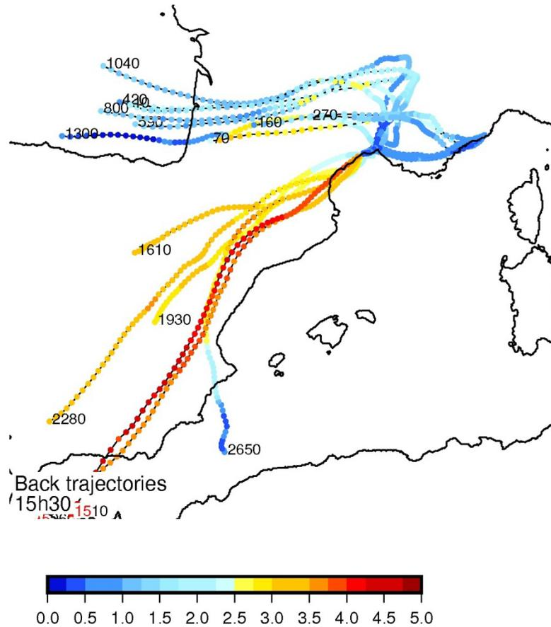
Air masses within the lower of the two upper layers are found to overpass Southern Spain and Morocco, descending from an elevation of 2-3.5 km, while air masses within the uppermost layer (up to 4 km) are not tracked by MESO-NH.
