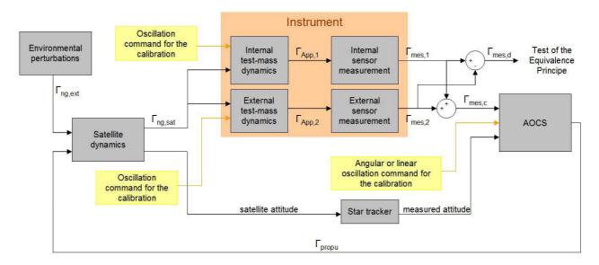
Fig. 1. The calibration simulator: the yellow blocks correspond to secondary inputs designed to oscillate the satellite or the test masses for the calibration.
