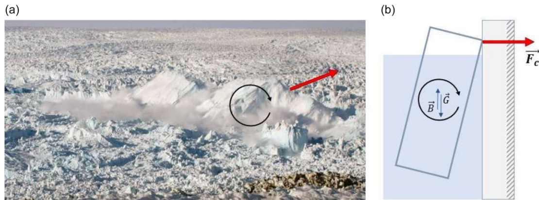
Figure 1. (a) Picture modified from Chasing Ice Calving by Jeff Orlowski showing an event occurring on 28 May 2008 at Jakobshavn Isbrae. The black arrow represents the rotation of the detaching iceberg. The red arrow represents the force applied on the terminus. (b) Schematic side representation of the phenomenon where buoyancy and gravity forces are represented with blue arrows.
