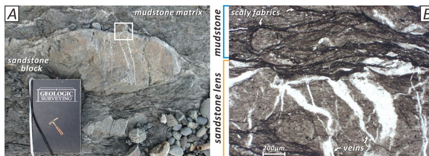
Figure 1. (a) Field photo showing the block-in-matrix texture of the Okitsu mélange in the Cretaceous Shimanto belt, Japan. (b) Photomicrograph of the Mugi mélange in the Cretaceous Shimanto belt. An intricate network of anastomosing scaly fabrics develops in the mudstone, accompanied by mineral veins that are primarily found within the embedded sandstone lens and, to a lesser extent, in the matrix.
