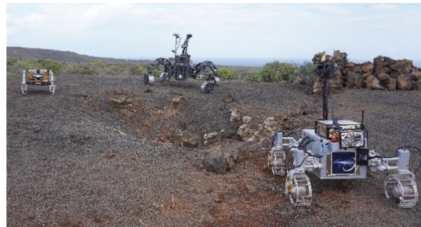
Figure 1 All three robotic explorer units involved in the field tests in Lanzarote surrounding the entrance to the subsurface lava tube, namely CoyoteIII, SherpaTT and LUVMI-X from left to right.
