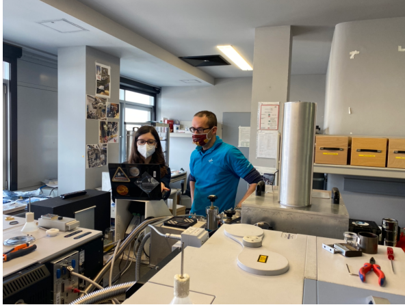
Figure 2. The VEM prototype during measurements at PSL to verify the instrument performance using Venus analogs at Venus surface temperatures
