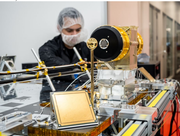
Figure 6: Gold Observatory’s instrument deck. Shown are the Planar Ion Probe (gold square), Floating Potential Probe (gold sphere & stick), Electrostatic Analyzer (gold & black cylindrical instrument), and multi-needle Langmuir probes (4 needles perpendicular to folded boom).
