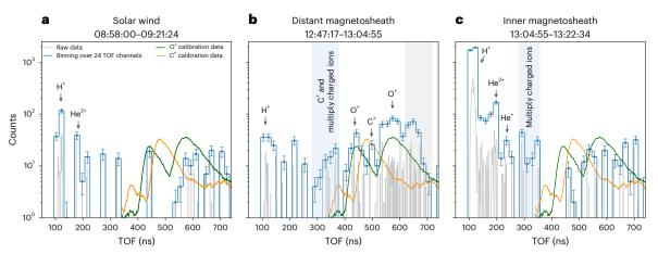
**Fig. 4** | **Three consecutive TOF spectra recorded during the second gravityassist manoeuvre of BepiColombo on 10 August 2021. a**, In the solar wind upon approach to Venus's induced magnetosphere. **b**,**c**, In Venus's induced magnetosheath in the time intervals 12:47–13:04 UT (**b**) and 13:04 UT–13:22 UT (**c**). The grey profiles show the data obtained using the full TOF resolution of MSA
