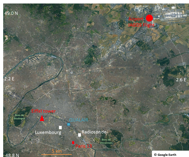
Figure 1. Google Earth map of the Paris area with O 3 and meteorological measurement positions during the ACROSS 2022 experiment. The blue mark is the position of the QUALAIR station including the O 3 DIAL (33 m a.s.l.) and instruments operated on the top of the Zamansky tower (125 m a.s.l.). The red triangle is the Eiffel Tower third platform (310 m a.s.l.), the red square is the AIRPARIF PARIS 13 in situ O 3 monitor in Parc de Choisy (50 m a.s.l.), and the red circle is the IAGOS aircraft take-off and landing airport. White squares show the Luxembourg park surface meteorological station (46 m) and the meteorological radiosounding station.
