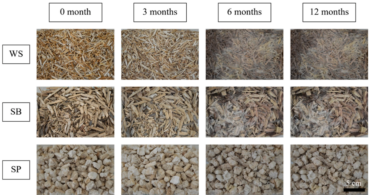
Fig. 4. Follow-up of microorganism development on rapeseed straw (RS), sunflower bark (SB), and sunflower pith (SP) at 0, 3, 6, and 12 months of microbial ageing.
