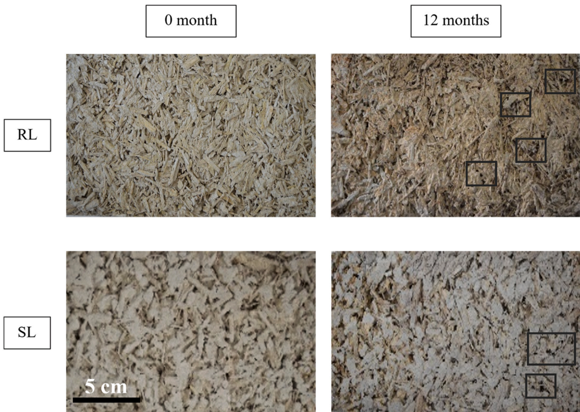
Fig. 5. Follow-up of microorganism development on the biocomposites RL and SL at 0 and 12 months of microbial ageing. Black boxes indicate the black dots of microorganisms developed on the surface of biocomposites.
