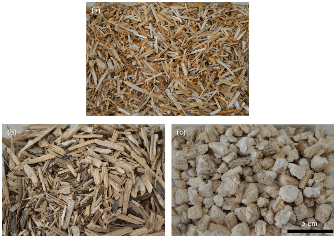
Fig. 1. Photos of the aggregates studied: (a) rapeseed straw (RS), (b) sunflower bark (SB), and (c) sunflower pith (SP) at 0 month before conservation conditioning.
