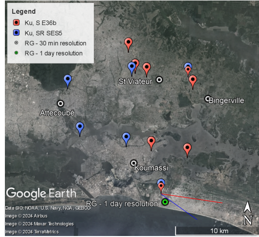
Figure 4. Map of available devices in the Abidjan area: Ku-sensors colored according to the satellite they target, E36b (red marker) and SES5 (blue marker); rain gauges represented by points with an enclosed circle: in white for the four 30-minute resolution rain gauges and in green for the Abidjan airport rain gauge at 1-day resolution (From © Google Earth Pro).
