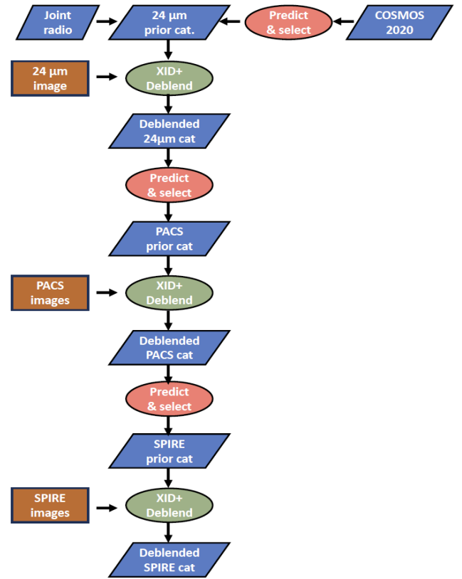
Fig. 4. Flowchart of our progressive deblending from 24 \mu\text{m} to the sub-mm wavelengths. Our initial prior catalogue for deblending the 24 \mu\text{m} map is constructed using COSMOS2020 and additional radio sources from the VLA-COSMOS 3 GHz and MIGHTEE 1.3 GHz catalogues. At each step of the deblending, we use a DLNN trained on an SED library to predict the fluxes of the sources in the prior catalogue at the relevant wavelength. Based on the predicted flux, we decide whether to keep the source in the prior list.
