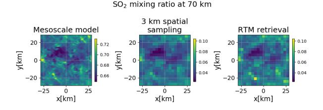
Figure 1: maps of the  $SO_2$  mixing ratio (RTM parameter): - simulated with the mesoscale model (left) - original map averaged to reach a 3 km spatial sampling, with rescaled values to be consistent with observed ranges (centre) - retrieved by the inverse RTM (right)
