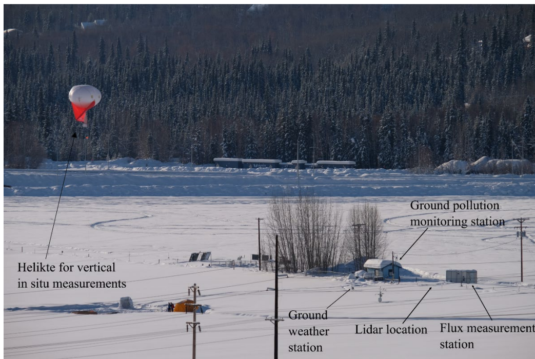
Figure 2 Photo of the UAF farm study site with the different infrastructures for ground-based and vertical measurements.
