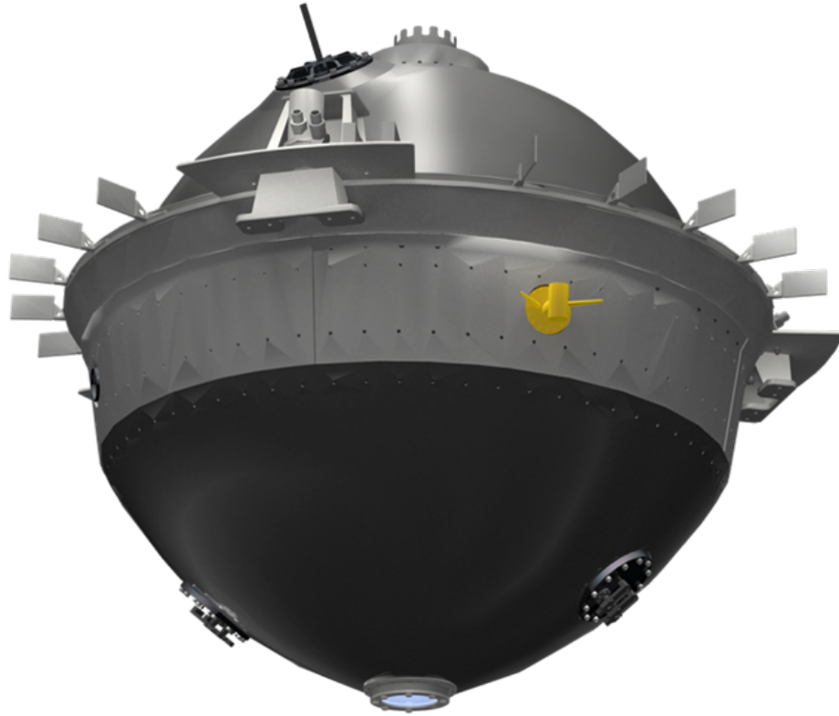
Figure 7: The titanium DAVINCI descent sphere, approx. 1 m diameter, protects its instruments from the extreme Venusian environment.
