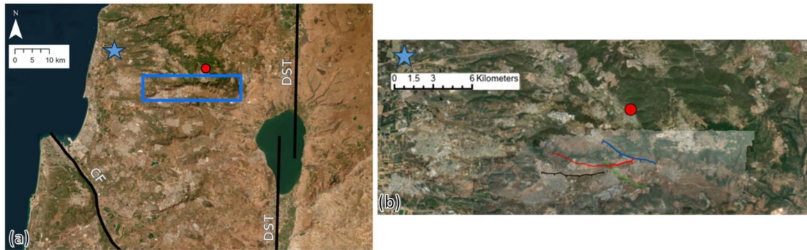
Figure 7. (a) The location of Kabri castle (blue star) relative to the Bet-Kerem fault system (blue triangle), the Dead Sea Transform (DST), and the Carmel Fault (CF). (b) Zoom in on the Bet-Kerem fault system, showing the location of the faults, outlined by colored lines: blue = Sajur segment, green = Nahf East segment, black = Deir Al-Assad segment, and red = Nahf segment, relative to the location of Peki'in cave (red point) and Kabri castle (blue star).
