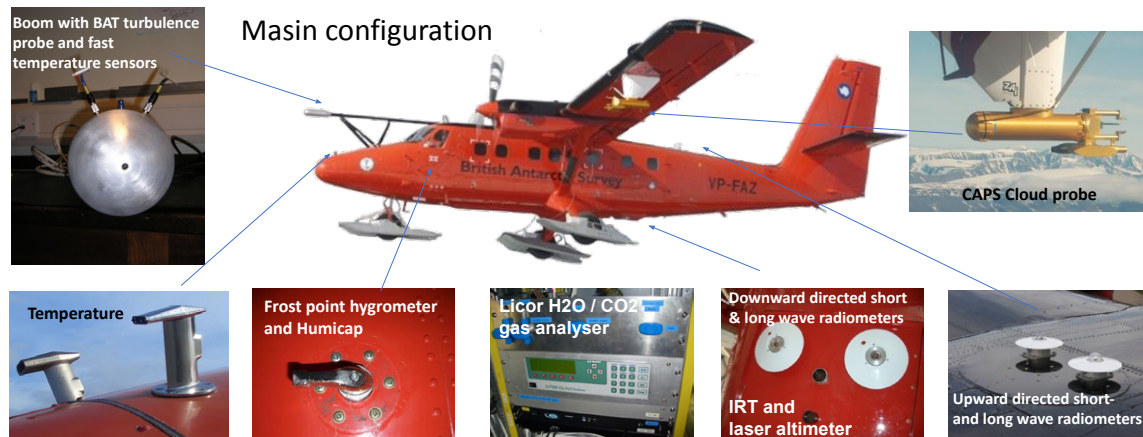
FIG. 2. Schematic of the BAS Twin Otter aircraft with the MASIN instrumentation. Acronyms are defined in Table 2.
