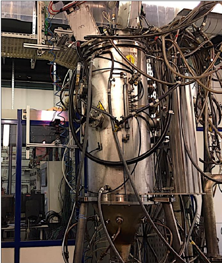
82 Fig. 1: a) 240kW three electrode arc plasma torch (PERSEE, Mines ParisTech, Sofia- 83 Antipolis, Nice) in which 600 g of a 20 \mu\text{m} -sized powder of NWA869 ordinary chondrite 84 have been processed for an hour. b) Simulated 3D thermal regime inside the condensation 85 chamber using the ANSYS Fluent computational fluid dynamic software. A removable T- 86 shape graphite rod was placed at the center of the chamber and was recovered after the 87 experiment for chemical and mineralogical analyses of the condensates. The 3D simulation 88 was performed in a computational domain that does not explicitly incorporate the T-shape 89 graphite rod. To account for the rod's presence, the torch power was set to the 90 experimentally determined value, maintaining the appropriate source temperature while 91 ensuring overall energy balance. To achieve this, losses induced by the rod were 92 redistributed onto the walls of the chamber, preserving the global thermal behavior of the 93 gas flow. While the thermal distribution may not be locally exact near the rod location, the 94 rod temperature can be considered to lie within the thermal boundary layer that forms near 95 the walls. Equivalence calculations suggest that the rod temperature is approximately 96 between 1/8 and 1/6 of the nozzle diameter away from the walls. 97
