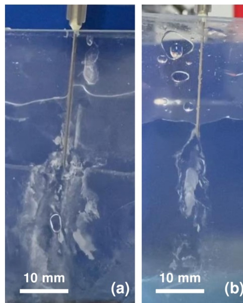
Figure 3. Two brinicle experiments 10 s after injection (a) and (b), following the 2D cell method with a 1 mm separation between the cell walls. In both cases solid instead of tubular ice structures were formed. See movie S1 in https://doi.org/10.20350/digitalCSIC/15364 (Testón-Martínez et al., 2023).
