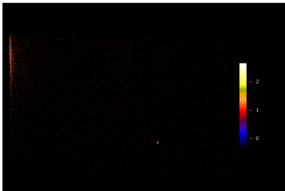
Fig. 22 Image histogram of the dark pixellist exposures for 16.7 hours of accumulated exposure. The color bar represents total counts in a given pixel over the accumulated exposure
