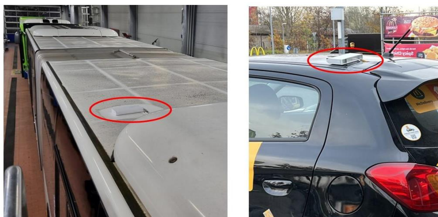
Figure 2. Pollutrack sensors (inside the red circle) on the roof of a bus (left) and of a car (right).
