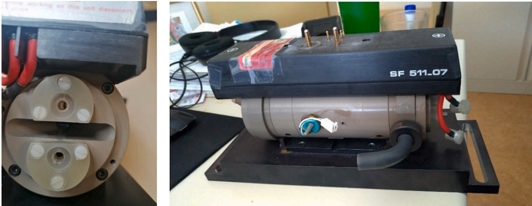
Fig. 1. Front and side vues of MEO A0 amplifier (with cracked flashlamp connectors).
