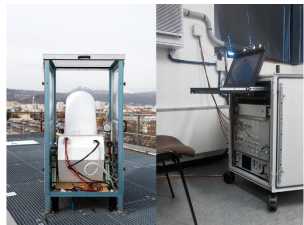
Figure 1: Optical (left, © Cyril Fresillon) and electronic (right © Jean-Luc Baray) parts of the LIDAR system.
