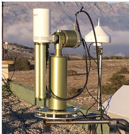
Figure 5. Cimel CE-318-TL9 photometer installed on Calern Observatory.
