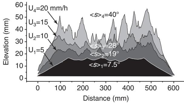
**Fig. 1** Effect of uplift on the local slopes and the local relief of steady-state topographies. The transversal topographic profiles are parallel to the length of the models, at a distance of 110 mm from the border of the uplifted zone. The mean local slope and the local relief increase with the uplift rate.  $U$ : uplift rate;  $\langle s \rangle$ : mean local slope.
