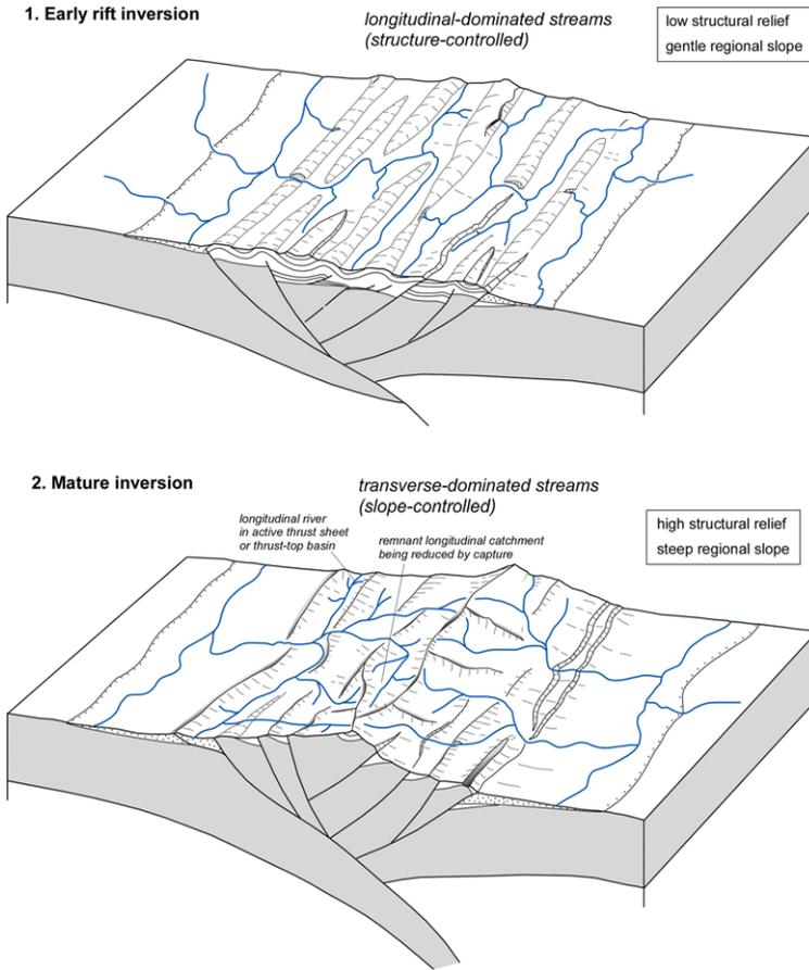
**Fig. 7.** Two-stage sketch model for the evolution of the drainage network in the Atlas Mountains of Morocco, modified after Babault *et al.* (2012), which can be of general application to inversion orogens which experience progressive increase of tectonic thickening and regional topographic slope.
