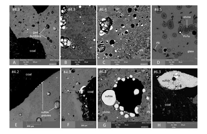
Fig.4.1. BSE images of experimental samples with coal addition. Experimental temperature and pressure are 1200°C and 75±7 MPa. The experimental duration is 10 minutes for (a), (b), (e) and (f), and 145 minutes for (c), (d), (g) and (h). Sulf: sulfide globule; cpx: clinopyroxene; plg: plagioclase; ol: olivine; coal: coal residues; Pt-Fe: Pt-Fe alloys. From Iacono-Marziano et al. submitted.
