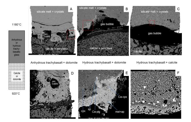
Fig.2.1 Magma-carbonate interaction experiments performed at ~200 MPa for a duration of 6 hours. A thermal gradient was imposed in the vessel to have a temperature of 1180°C at the top of the sample and 920°C at the bottom. (A), (B), (C) BSE images of the central part of the capsule where the interaction is maximum. (D), (E), (F) Zoomed-in BSE images of the red squares in (A), (B), and (C).
