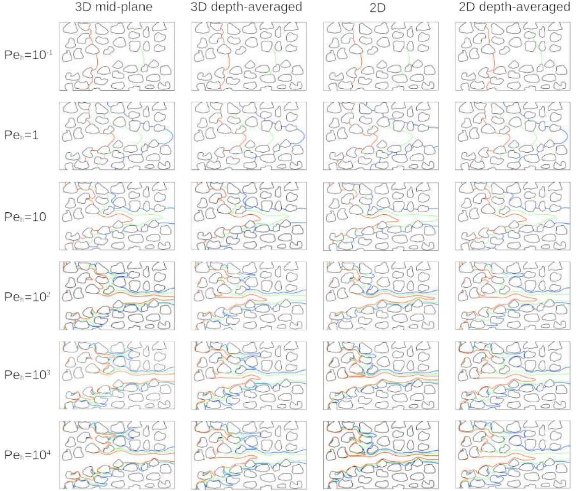
Figure 5.3: Transport of a scalar in a micromodel with aspect ratio h/d > 1 . We use 3D, 2D and 2D-depth-averaged models for different Péclet number by varying the diffusion. The results correspond to isocontour of the concentration for C = 0.2 (blue), C = 0.5 (green), C = 0.8 (orange) at t = 42 s. 2D models without dispersion break down for Pe_h > 10 (from Soulaïne et al. (2021b)).
